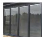
GL-1 High performance double glazing system U Value Max 2.5 w/m2K Colour: Clear SHGC 0.3
